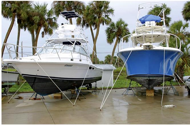
**Left:** Boats that are hauled out are far less likely to be damaged during a storm than those left in the water. Using straps is effective at keeping boats from toppling over or floating away. **Below:** Lines should be extra long to allow for surge. Double up lines where possible.
